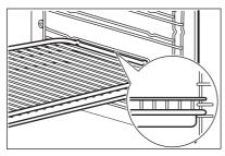
Small indentation at the top i increase safety. The indentations are also anti-tip devices. The high rim around the shelf prevents cookware from slipping.
