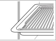
**2.** Put the deep pan into the oven on the necessary shelf position.
