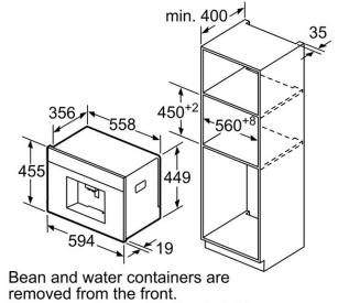
Recommended installation height 95-145 cm. measurements in mm
