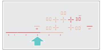
The function has now been activated. The Lerr temperature symbol flashes until the frying temperature is reached. A signal sounds and the temperature symbol goes out.
