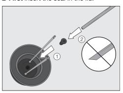
Make sure you do **not** fit the slanted end of the milk intake tube into the seal. This would damage it.
