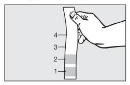
Dip the test strip in your drinking water for approximately one second, then shake off any excess water. The result will be evident after about a minute.
