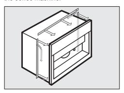
If the housing unit niche is not fitted with a sealing strip, you should fit a Miele sealing strip to the machine before installing it. This is fitted from the back of the machine.
