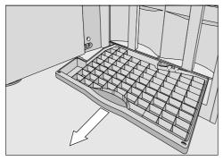
Open the machine door and carefully remove the drip tray from the machine.
