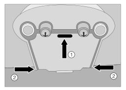
■ To remove the sensor cover, press and hold the cover ① between the two dispensing spouts. Then press the sides of the central spout ② at the back.
