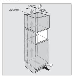
Air intake ① occurs via the plinth at the bottom of the machine and the air escapes at the top ② at the rear of the housing unit.
