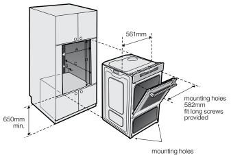
mounting holes fit countersunk screws with plastic spacers provided
