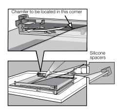
Insert the remaining smaller clear glass panel into the middle position, ensuring the chamfered corner of the panel is placed in the correct location as shown in the image below.
