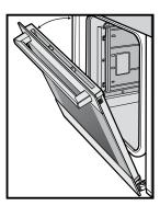
• Grasp the oven door with a hand each side of the door and remove it from the oven by pulling it towards you.
