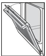
• Hold the oven door with a hand each side and remove it from the oven by pulling it towards you.
