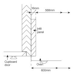
Note: Your appliance must be mounted on a flat surface for the full width and depth of the product
