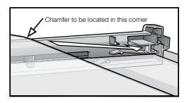
• Insert the black bordered glass panel into the upper position, ensuring the painted surface is facing the downside as per the image below.
