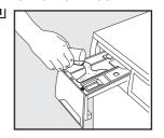
If required, pour fabric softener into the compartment marked & (the amount used must not exceed the "MAX" mark in the drawer).
