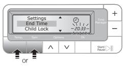
Press the Start/Pause button to start the programmes will start after the selected delay has expired.
