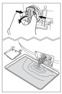
When the container is full of water, put the drainage duct back again and empty the container. Do step 3 again and again until no more water flows out from the drain pump.
