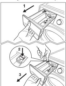
To aid cleaning, the top part of the additive compartment should be removed.
