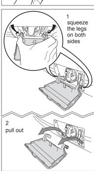
Place a suitable water container below the recess of the drain pump to collect the water that flows out.
