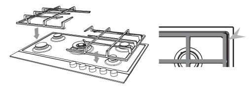
Correct positioning of pan supports (CG905DX models)
