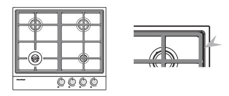
Correct positioning of pan supports (CG604DX models)
