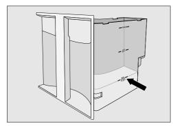
■ Fill the water container to the //|\\ marker with lukewarm water and stir the solution.
