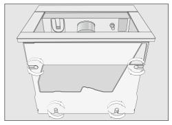
■ Using the large allen key, unscrew all four feet out by about 2 mm.
