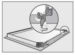
■ Then refit the upper of the middle two panes in such a way that the material number is legible (i.e. not reversed). The glass pane should lie on top of the retainers.
