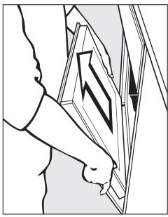
Hold the door securely at both sides, and lift it upwards off the retainers. Make sure you take it off straight.
