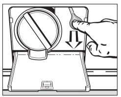
Pull the emergency release downwards (see illustration). The drum door will open. In the event of any faults which you cannot remedy yourself, please contact Miele (see back cover for contact details).
