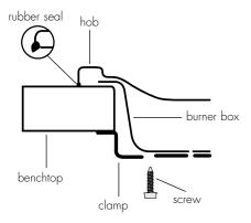
• Fit the pull-down clamps supplied to ensure that the cooktop cannot move after installation.
