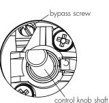
(<del>(((())))</del>) flame size adjusted to maximum
